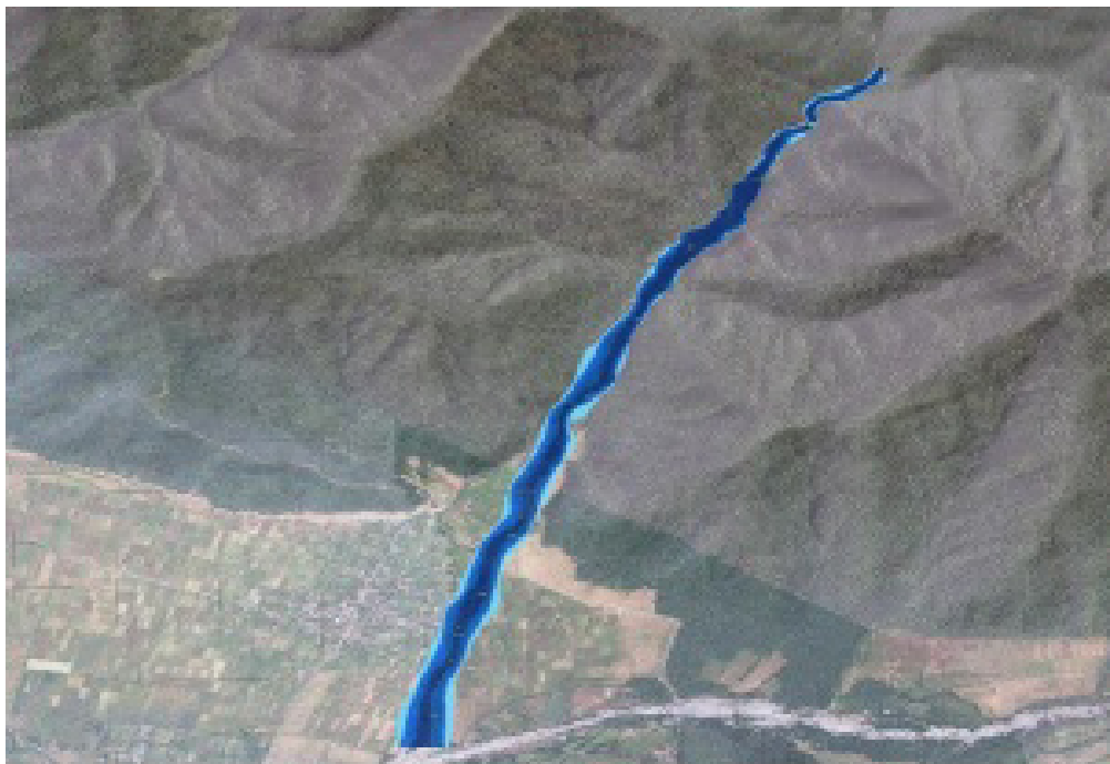
Figure 24. Modeled Flood Hazard Map of the Duruji River (NEA, 2015).
